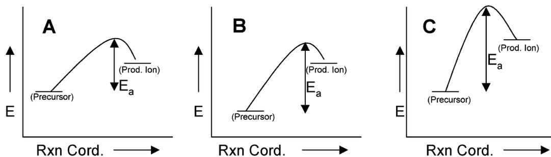
Figure 1. Energy level diagrams for three dissociation reactions. (A) Dissociation with low activation energy. (B) Dissociation with higher energy barrier: Precursor is stabilized relative to the transition state. (C) Dissociation with high energy barrier: Product is high in energy.
