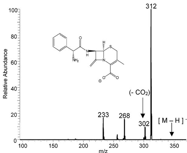
Figure 6. MS/MS of cephalixin. Loss of carbon dioxide was incorrectly predicted due to a lack of information on the effects of the amide. Carbon dioxide loss ( $m/z$  302) has a low abundance of  $\sim 9\%$ .
