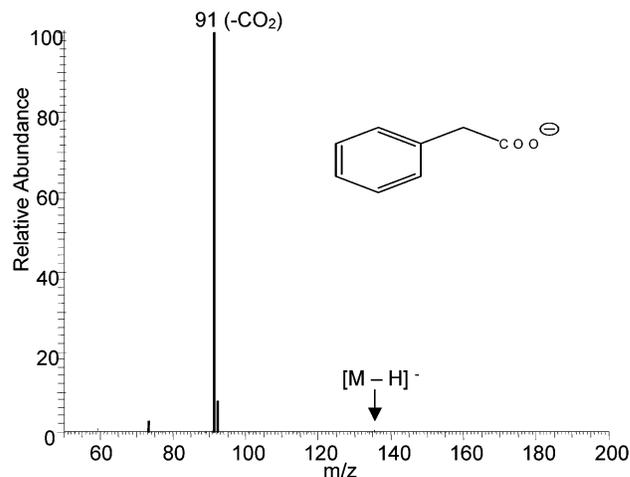
Figure 3. MS/MS of phenylacetic acid (**1**). The predominant product ion, *m/z* 91, corresponds to a neutral loss of CO<sub>2</sub>.
